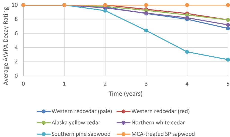
Figure 2: Average Extent of Decay in Test Materials Exposed in Saucier, Mississippi.
