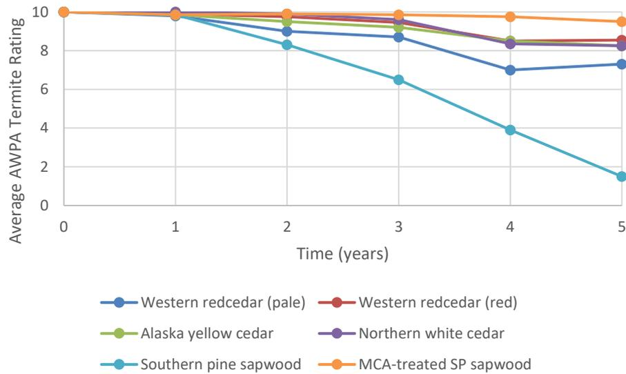
Figure 4: Average Extent of Termite Attack in Test Materials Exposed in Saucier, Mississippi.
