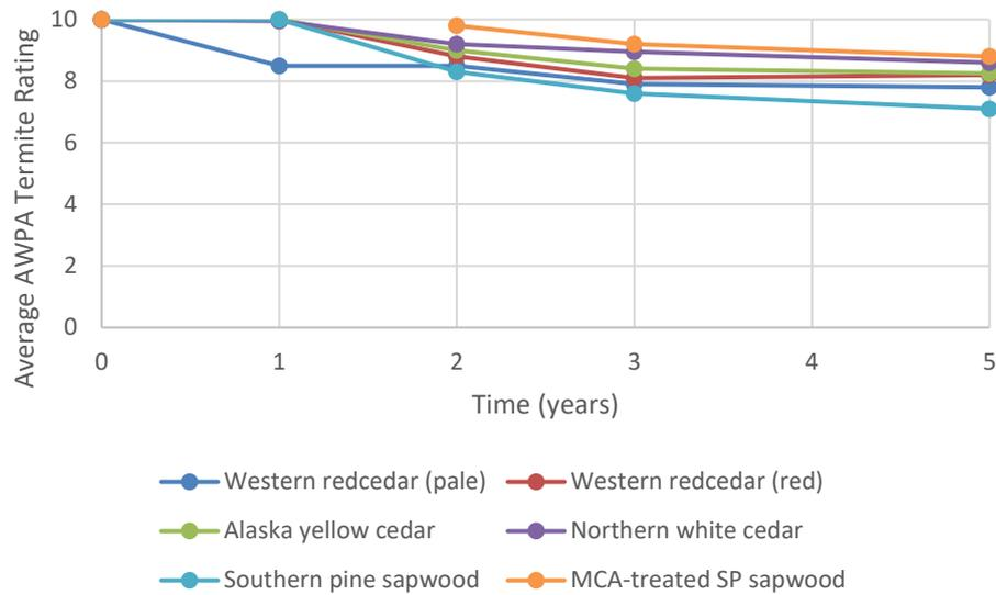
Figure 3: Average Extent of Termite Attack in Test Materials Exposed in Kincardine, Ontario.
