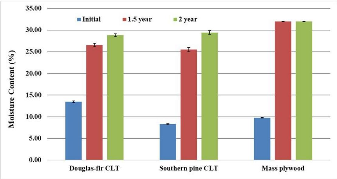
Figure 6: Average surface moisture content of mass timber samples (n = 120) at test initiation, then after 1.5, and 2 years of exposure in an above-ground protected field test in Saucier, Mississippi USA.
