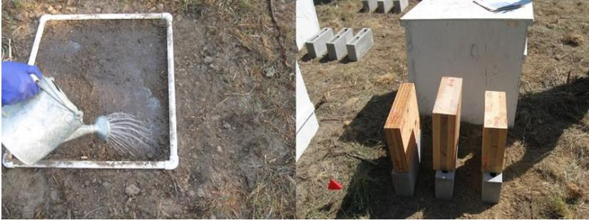
Figure 2: Drench treatment with fipronil soil termiticide and arrangement of ground bricks and CLT in soil termiticide subplots before covering. Note the hand tilled soil. PVC frame used as guide for insecticide application.
