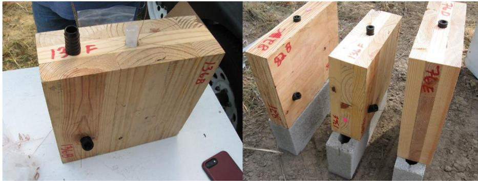
Figure 4: Arrangement of blocks and samples for boron rod treatment. Two rods placed in each sample at top and one face (left). Samples with rods capped, placed on blocks and covered (right).
