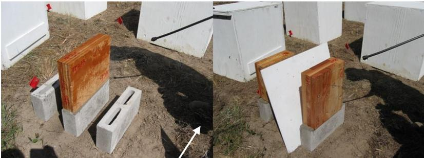
Figure 3: Arrangement of blocks and samples in subplots for preventive and remedial treatments sprayed with borate solution (23% DOT) before cover was placed over samples (note plastic barrier to minimize drift on adjacent samples).
