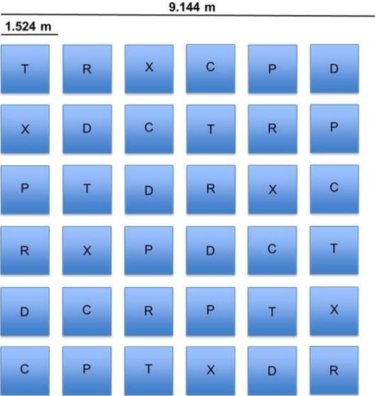
Figure 1: Layout of randomized block design for the modified AWPA E21 ground proximity field test. P = Protective treatment with borate (DOT at 23%). T = Treatment with fipronil soil termiticide (0.125%). C = Control. R = Remedial borate spray treatment (23% DOT) after two year check. D = boron rods in samples at initiation. X = Subplot not used.
