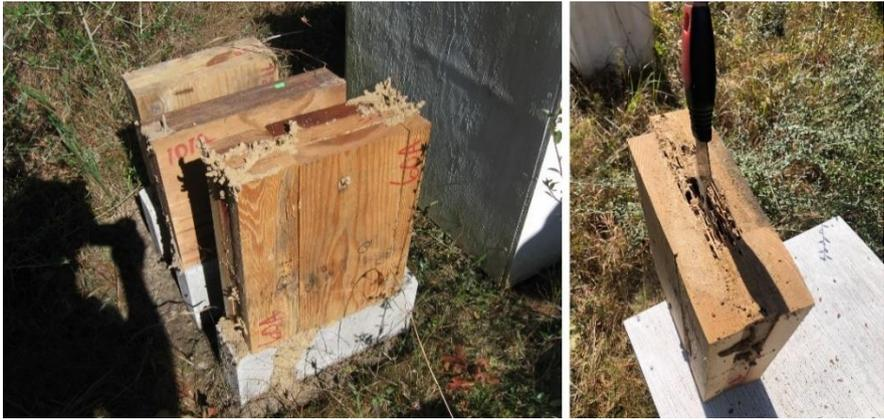
Figure 7: Examples of termite attack showing extensive mud tubes on a Douglas-fir CLT sample (left) and termite tunnelling and excavation underneath the sample at the two-year rating (right).
