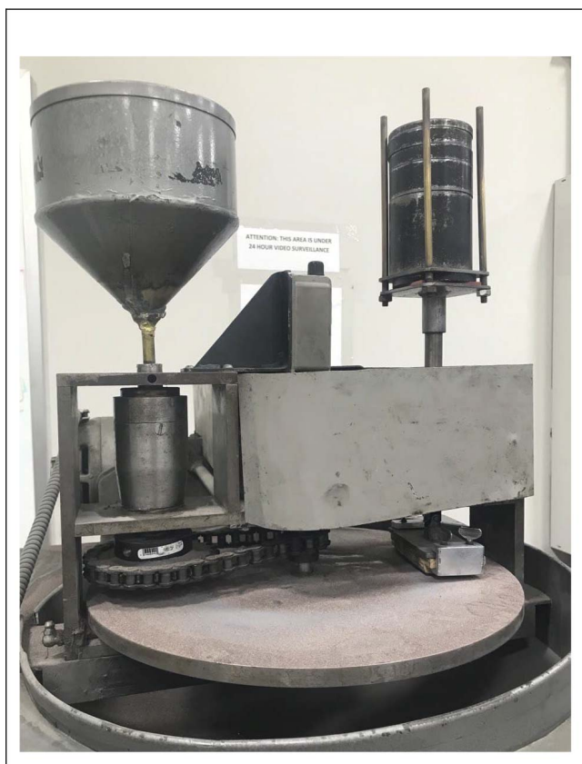
Figure 2.—Navy-type wear tester used to conduct abrasion test.
