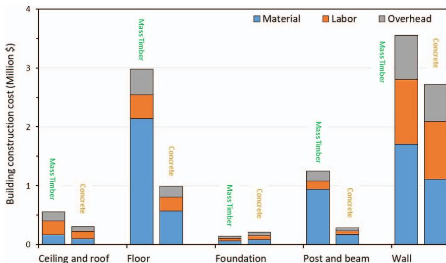
Figure 1.—Front-end construction costs by assembly type for high-rise mass timber and concrete buildings.
