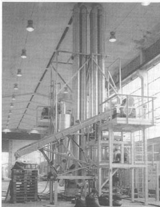
**Figure 22.2.** Fiber acetylation pilot plant in Sweden
