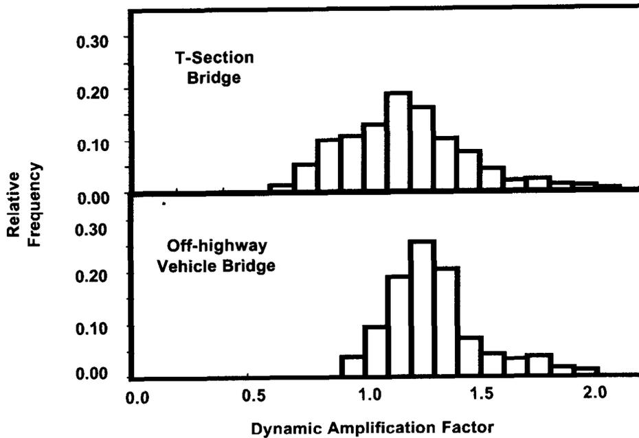
Figure 5. Relative frequency histograms of Dynamic Amplification Factors. All speeds and entrance conditions are included.
