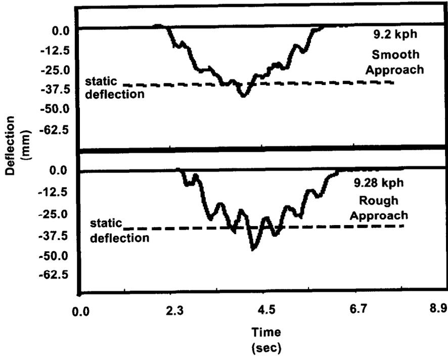
Figure 4. Typical deflection plots from dynamic load tests of the off-highway vehicle bridge.
