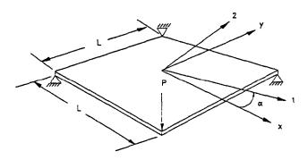
Figure 10 - Schematic of Pure Twisting Test Loading Geometry
