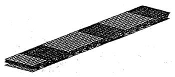
Figure 8 - Finite Element Mesh for MD Four Point Bending
