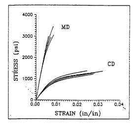
Figure 3 - Stress-Strain Curves (Tension, Liner)
