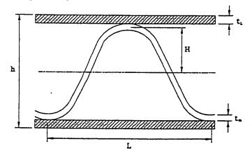
Figure 2 - Corrugated Board Key Dimensions
