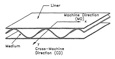
Figure 1- Corrugated Board Structure
