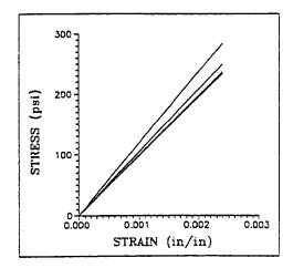
Figure 5 - Pure Shear Stress-Strain Curve Data (Liner)
