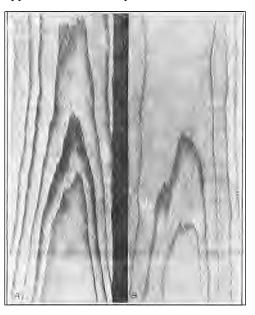
Fig. 8—A. Raised grain on the pith side of a white spruce board. B. The bark side of the same board, without raised grain.
