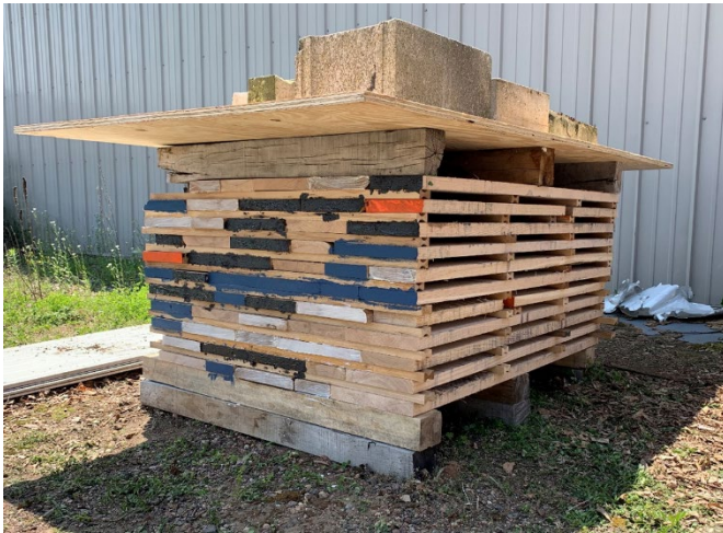
Figure 1—Randomly selected end coatings of air-drying lumber. Orange end coloring marks the boards that were used to monitor moisture content (similar in use to kiln samples in a kiln charge). Boards with black-colored ends were treated with roofing compound, blue-colored ends were treated with latex paint, and white-colored ends were treated with emulsified wax. Boards with no color added are the uncoated controls.
