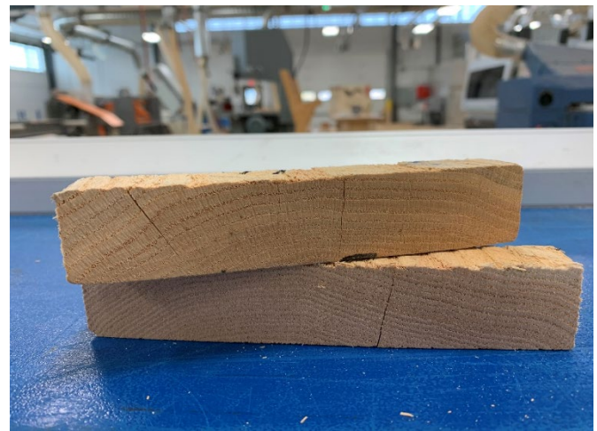
Figure 2—End splits resulting from rapid end drying. The splits are in the radial direction because the wood rays form planes of weakness.
