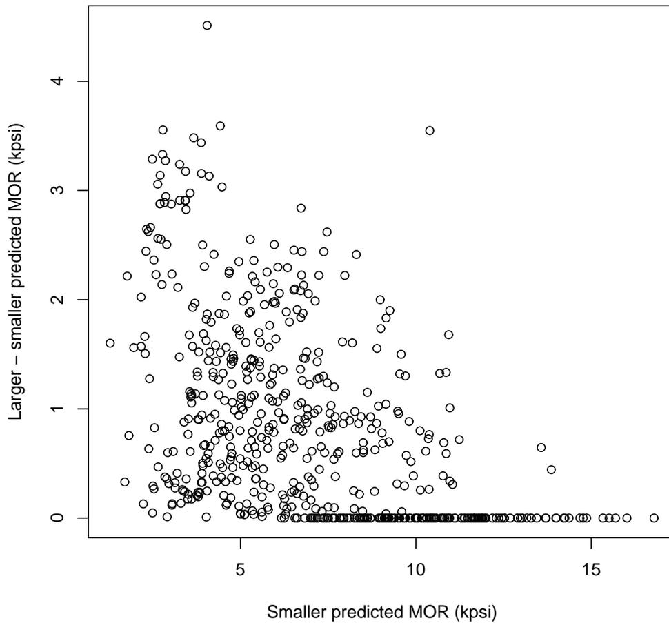
Figure 15: “Flipping a board” (exchanging compression and tension edges). Plot of larger minus (same board) smaller predicted strengths versus the smaller predicted strengths. Model 4.
