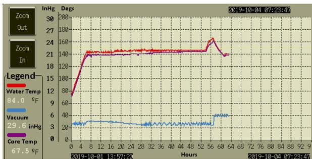
**Figure 3. Vacupress (Vacutherm, Inc., Barre, Vermont, USA) drying schedule, medium setting.**
