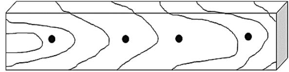
**Figure 4. Diagram showing best judgement sampling of clear areas on a tangential surface.**
