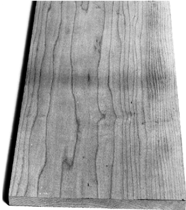
Figure 13–17. Sticker stain in sapwood of sugar maple after planing.
