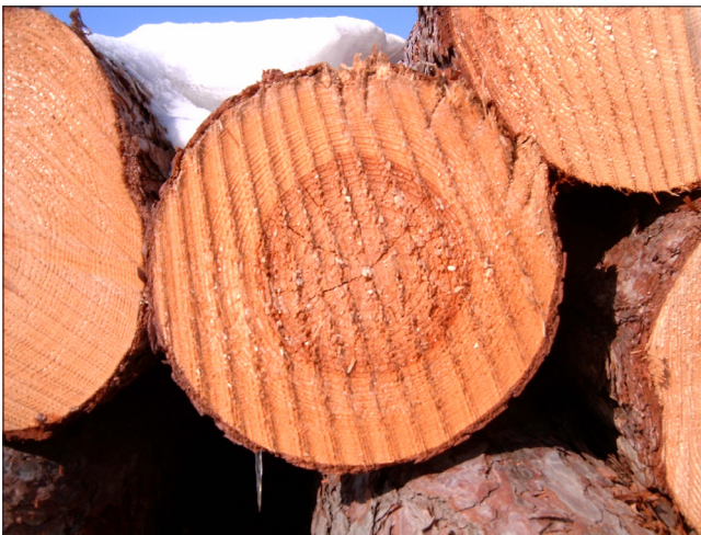
Figure 13–9. End checking in red pine logs.
