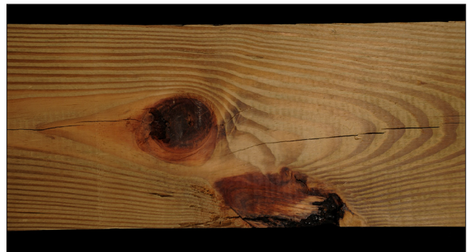
Figure 13–12. Large knot in treated Southern Pine.
