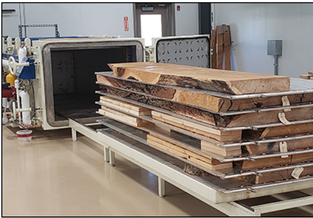
Figure 4. Charge of thick slabs stacked in single layers between heating platens.
