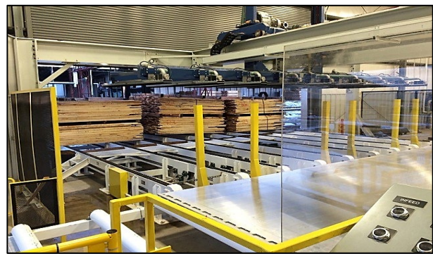
Figure 7. Mechanized, automated loading system at a large-scale drying operation (photo used with permission from Vacutherm, Inc., Barre, Vermont, USA).
