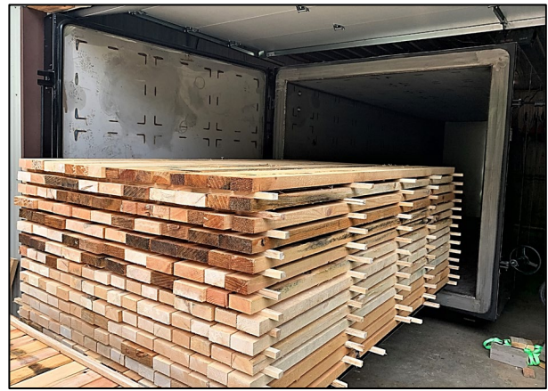
Figure 6. Charge of lumber hand-loaded and stickered for drying in a cyclical vacuum kiln.
