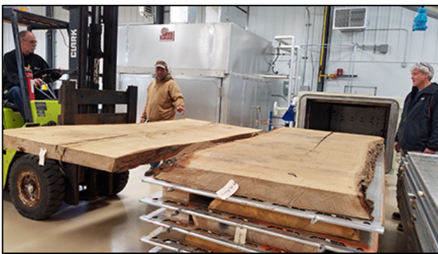
Figure 5. Loading 4-in.-thick white oak live-edge slabs into a vacuum kiln. These large slabs require the use of a forklift for the slabs and hand-loading of the aluminum platens between each slab.
